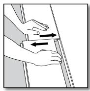
**[14]** The released planks can then be pulled apart by sliding them out horizontally. Never bend connected planks downwards; this will damage the planks' locking ridges.
