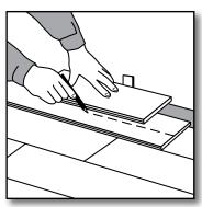
[16] Use a full width scrap plank to mark your cutting line on the last row.
