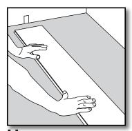
[1] Assemble three or four rows well away from the starting wall. Begin by placing the tongue of the short plank toward the starting wall.
