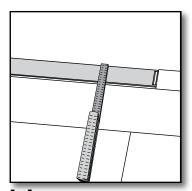
[15] Measure and cut the planks in the last row to fit. Remember to allow for a minimum of 1/4" expansion space from the wall.
