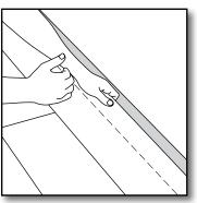
[12] To remove the first row for cutting, lift the planks a few inches and tap along the joint. Cut the planks as required. Re-connect all of the first row end seams and replace the first row by pressing the first row into place with the groove toward the edge of the planks that are already in position.
