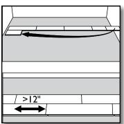
**[5]** Use a cut piece of board from the previous row to start the next row. This starting plank section must be at least 12" long. If the piece is too short, start with a new board. Cut the new board in one-third, one-half or two thirds length sections, depending upon what is required to maintain the random stagger from one row to the next. Always ensure that the end joints are staggered at least 12 to 16 inches from one row to the next.
