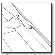
**[12]** To remove the first row for cutting, lift the planks a few inches and tap along the joint. Cut the planks as required. Re-connect all of the first row end seams and replace the first row by pressing the first row into place with the groove toward the edge of the planks that are already in position.
