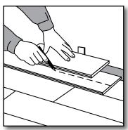
[16] Use a full width scrap plank to mark your cutting line on the last row.
