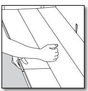
[13] You may have to disassemble the flooring due to obstructions, etc. Just lift the row of planks a few inches and tap along the joint.
