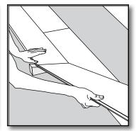
[7] Attach the second plank of the second row to the first planks end seam; but again, do not fold these planks down into the locked position. You can easily construct wood wedges to help hold these planks in place in the unlocked position (see diagram).
