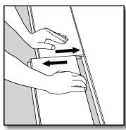
**[14]** The released planks can then be pulled apart by sliding them out horizontally. Never bend connected planks downwards; this will damage the planks' locking ridges.
